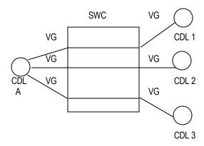
The customer requests the installation of a DS1 between the serving wire center (SWC) and CDL A and a DS1/voice multiplexer in the SWC. The customer also requests that the voiceband circuits serving CDLs 1, 2 and 3 be "rolled over" to the new DS1. All NRCs apply for the installation of the DS1 and multiplexer. No NRCs apply for the voiceband rollovers to the new high capacity circuit.
