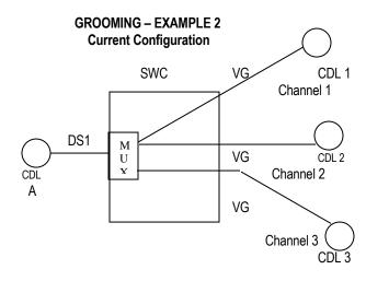
The customer requests that the voiceband circuit serving CDL 3 be moved from channel 20 in the DS1 serving CDL A to Channel 3 in the same DS1. No NRCs apply for this request.
