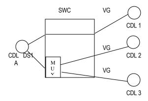
The customer requests that the voiceband circuit (VG) between CDL A and CDL 1 be "rolled over" to the DS1 servingCDL A. No NRCs apply for this request.
