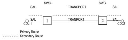
Two diverse circuits between serving wire centers. The SAL and Transport facilities must be separate, although the SWC's may be the same.
