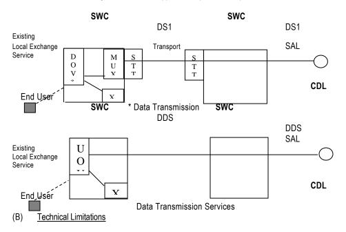
Data Transmission Services service operates over two-wire non-loaded copper facilities and is subject to a maximum cable length of 18,000 feet.
