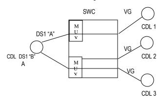
The customer requests that the voiceband (VG) circuit serving CDL 1 be moved from the DS1 "A" circuit to the DS1 "B" circuit. No NRCs apply for this request.
